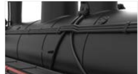
Separately attached boiler pipes
