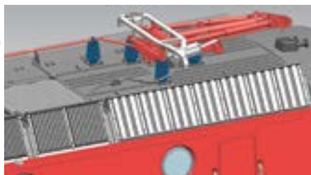
Separately applied cable to the current collectors
