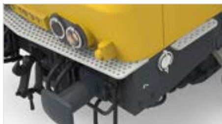
Running boards made from perforated metal
