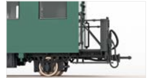
Platform area features almost-invisible coupling mounting
