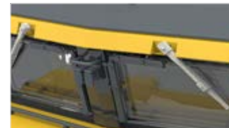
Plug-in windshield wipers and sockets
