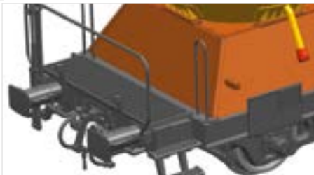
Detailed shunting platform with perforated grid
